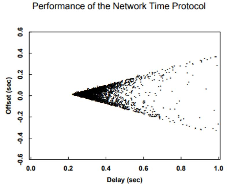
Figure 3. Offset vs Delay
