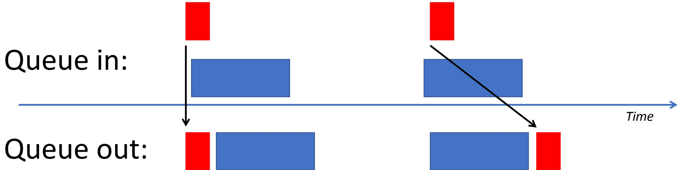
The Maximum QOS priority inversion delay is the *output port wire speed time of a full size packet* multiplied by the *number of switches* the high priority packet passes through.
