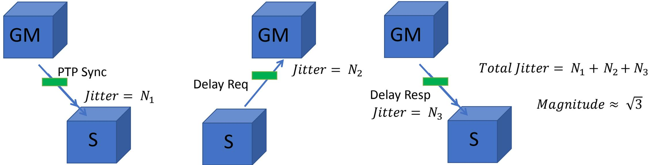
An audio clock recovered from PTP using peer delay will be less stable than an audio clock recovered from only the PTP sync packets.
