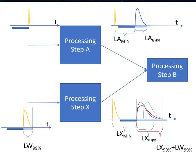
Variability on the input accumulates into the output!!!
